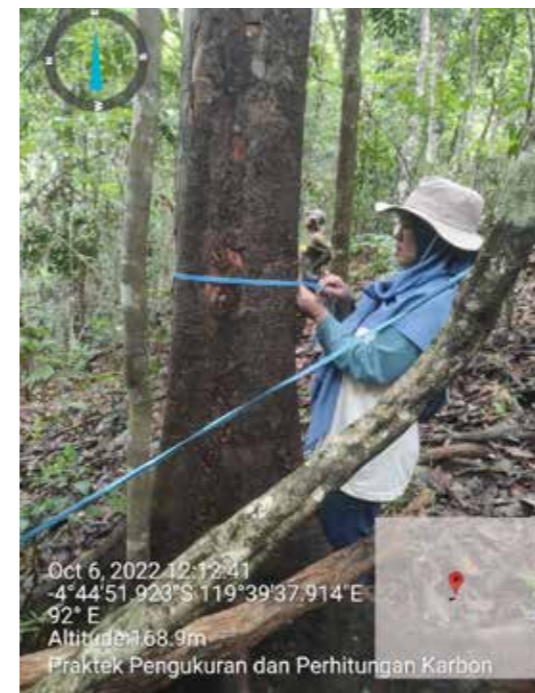
Measuring the tree diameter at breast height (DBH) during the capacity building and training on accounting of carbon stocks and emissions reduction for FMU officers in South Sulawesi Province, Tabo-tabo Forest Area with Specific Purposes, South Sulawesi Province, Indonesia
