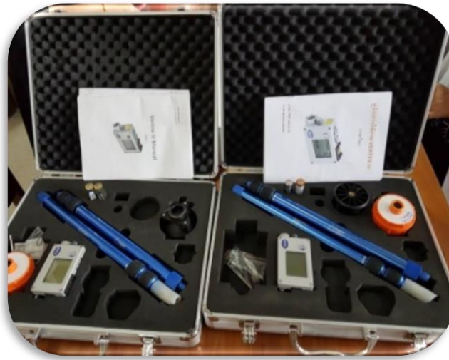
Figure 43: 2 sets of height meter were purchased. Height meter (vertex) (Haglof VERTEX IV)
